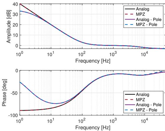
**Figure 3: Results obtained with CCIR 30ips recording curve and NAB 15ips reproducing curve. It is possible to notice that the pole translation does not cause evident problems in the digitization of the transfer function.**
